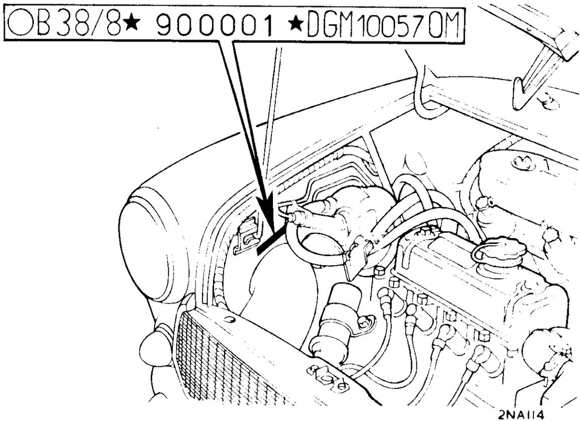
The **Car Number** and **Body Number** are stamped on a plate secured to the right-hand front wheel panel valance in the engine bay
