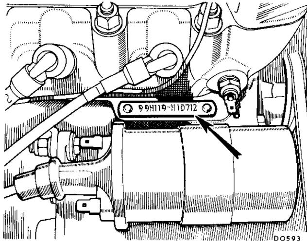
The **Engine Number** is stamped on a plate secured to the cylinder block
