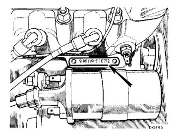
The Engine Number is stamped on a plate secured to the cylinder block
