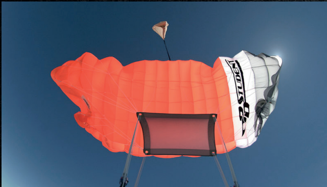
Closed end cells Attempt to air up the end cells by making a steering test
