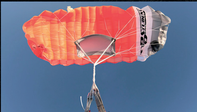
Line twists (fully inflated canopy) Attempt to clear twists, if not possible, emergency procedure
