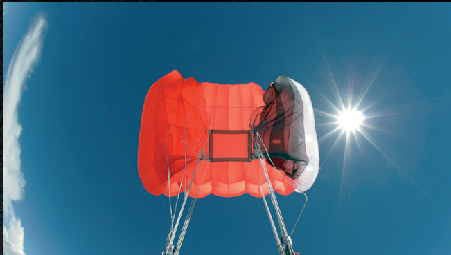
Line entanglements Emergency procedure
